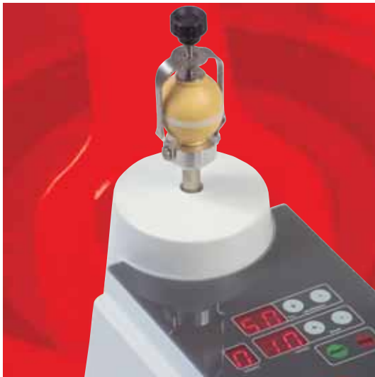
clamping system and integrated glass keyboard
