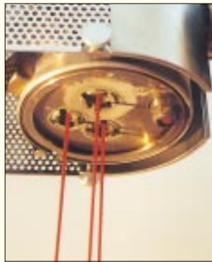
MBR-TD with three capillaries
